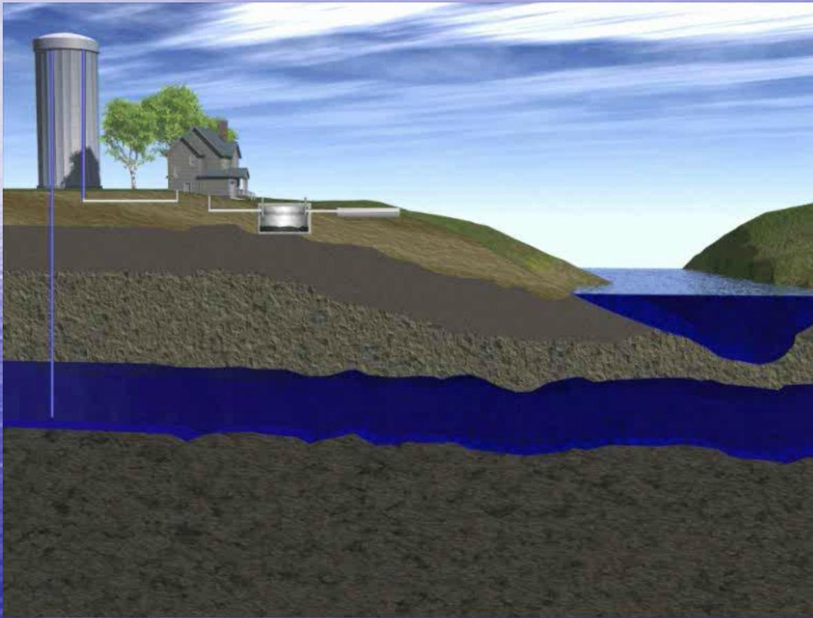
Groundwater is extracted from one point and delivered to multiple locations but still returned to the aquifer via onsite systems
